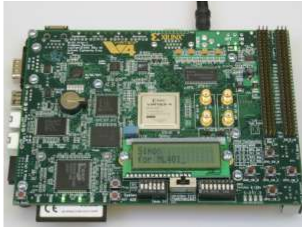
Figure 3: Xilinx ML401 Evaluation Board with Virtex 4 LX25[ 20 ]
